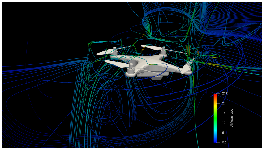
Figure 45: Velocity streamlines on the simplified overmount Dji Phantom 3.
