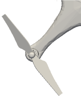
Figure 19: 1/4^{th} section of the quadcopter, used to assign patches for the MRF properties file .
